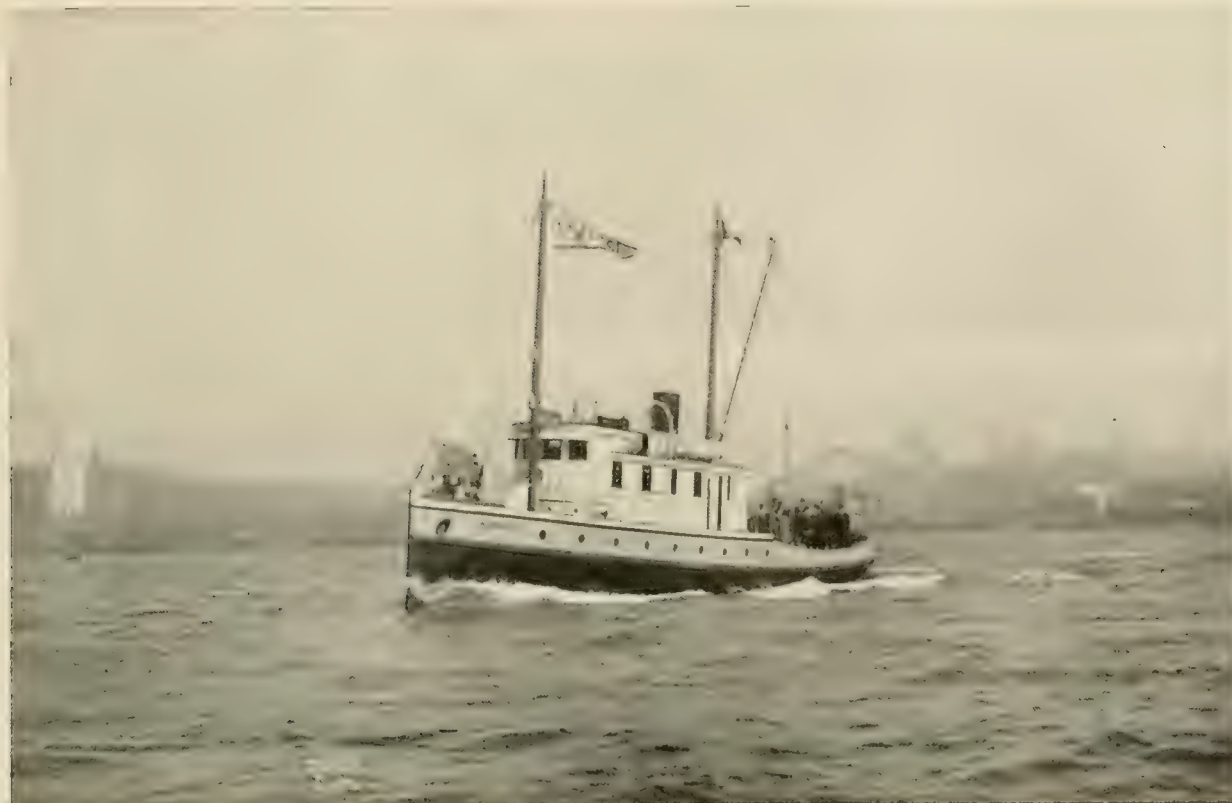
PACIFIC AMERICAN FISHERIES CANNERY TENDER WARRIOR. This is the First Cannery Tender to be Equipped With a Diesel Engine.
